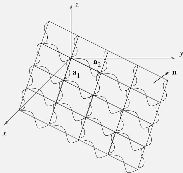
Figure ldr\_3d\_2p.1 Solution of Laplace's equation above a doubly periodic surface with arbitrary orientation subject to the Dirichlet boundary condition, computed by a boundary-element method based on the double-layer representation.
